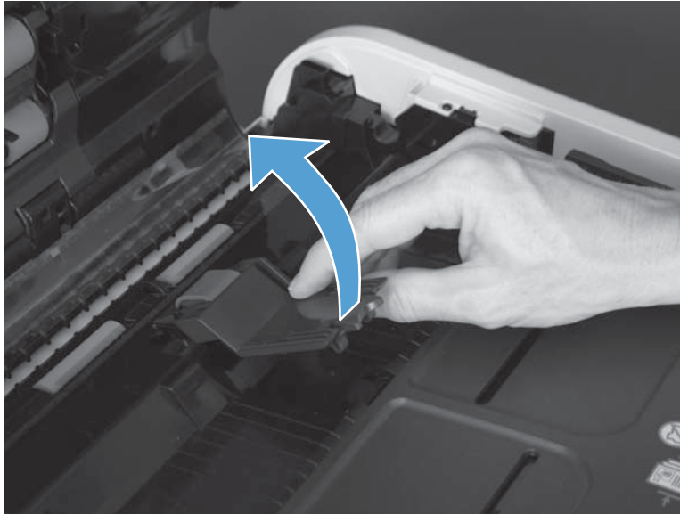
Figure 1-53 Remove the document feeder separation pad (3 of 3)
