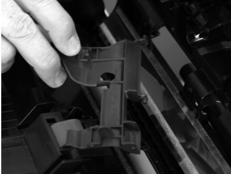
Figure 1-69 Remove the document feeder roller cover (4 of 4)
