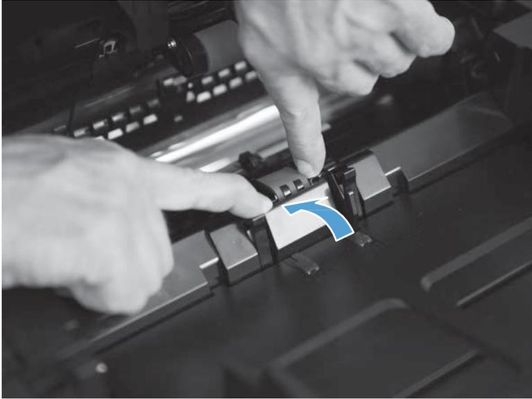
5. Verify that the separation pad is correctly installed and that the access door is fully closed as shown below.
