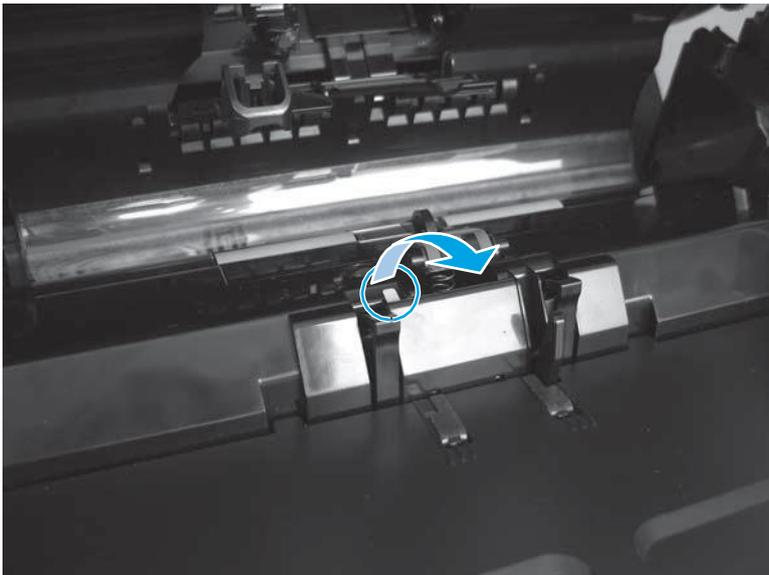
**3.** Hold the access door open to allow the separation pad to partially release and pop up.
