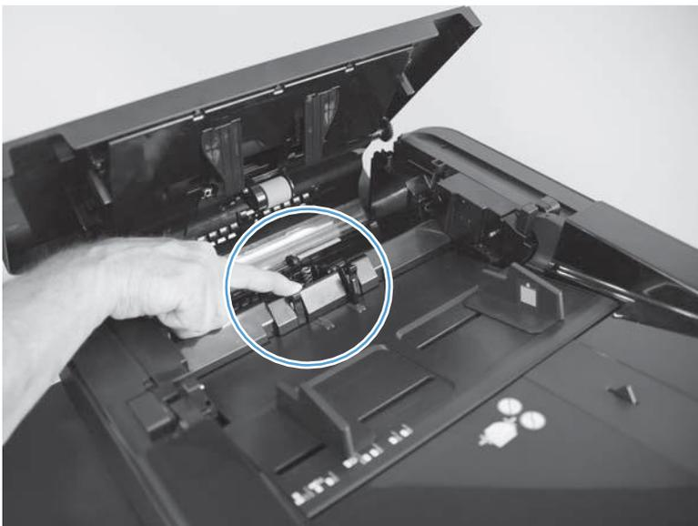
2. Align the pins on the separation pad with the mounting slots.
