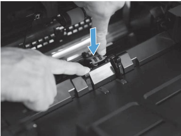
4. Continue to press down on the separation pad, and then release the access door.
