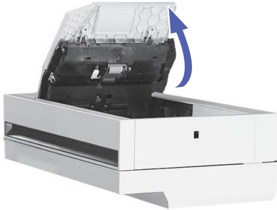
Figure 9-11 Open the document-feeder jam access door
